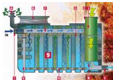
Figure 8 : Filtre compact (Source SEBICO)
